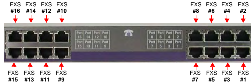
Figure 3: FXS Connectors Port Numbering Convention (Mediatrix 4108/4116)
