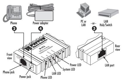
Figure 1. SmartLink M-ATA installation diagram
