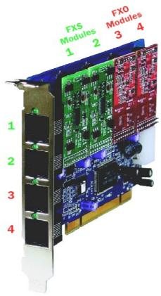
Notice how the modules are tied to the ports. The following picture shows the example of a TDM22B and how the port location corresponds to the module location
