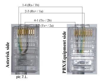
When connecting a NTPM, it is possible the wires are crossed inside the NTPM. In this case, use a simple patch cable (pin 1 to pin 1).
