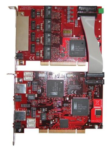
The order of the PCI cards is very important regarding the Master/Slave settings. The order is defined by how you have entered the PCI card into the Computer and how the mainboard has wired the PCI Slots. In general it is not known how the order will be.
