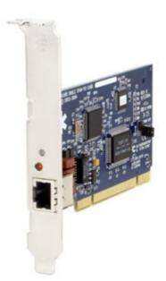
The TE110P (E100P, T100P) is a 1-Port T1/E1 card. The card has a jumper that lets you choose whether the card should work in the T1 or the E1 mode. Please set the jumper accordingly. This jumper is not present on the older, obsolete E100P and T100P cards because a different card exists for each mode. Install the card in an empty PCI slot and restart your system.
