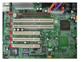
The **TE411P** is a 32-bit 33MHz card keyed for 3.3 volt operation. In the motherboard pictured here, the TE411P will **only** fit into slot #2. The TE411P **will not** fit into slots 1, 3, 4, or 5.
