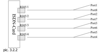
Each end of the Y-cable has an RJ45 jack. If you want to connect ISDN telephones, please use straight RJ45 cables.
