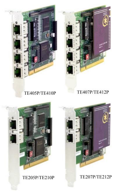
The TE4xxP (TE405P, TE406P, TE410P, TE411P) is a 4-Port T1/E1 card. The difference between the TE405P/TE410P and the TE406P/TE411P is that the TE406P/TE411P has an additional daughter board for hardware echo cancellation.
