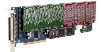
The TDM2400P is a mother board with space for a total of six analog modules. Each of the modules provides four analogue channels (4xFXO or 4xFXS). The following combinations are available:
