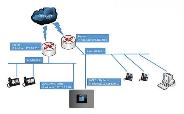
Figure 21: UCM6302 Network Interface Method: Dual
