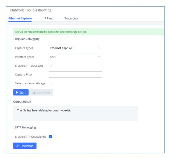
Figure 368: Ethernet Capture
