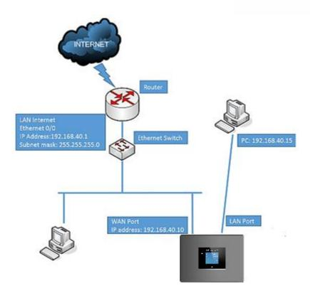
Figure 20: UCM6302 Network Interface Method: Switch
