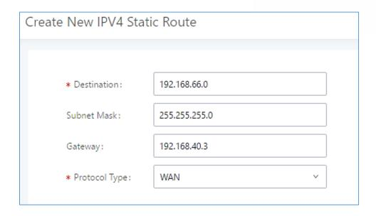
Figure 25: UCM6304 Static Route Configuration
