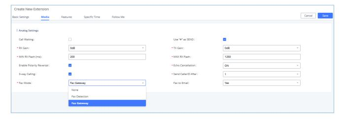
Figure 141: Configure Extension for Fax Machine: Analog Settings
