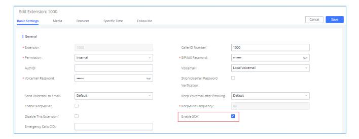
Figure 237: Enabling SCA option under Extension's Settings
