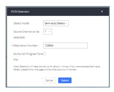
Figure 106: UCM630X PSTN Detection: Semi-Auto Detect
