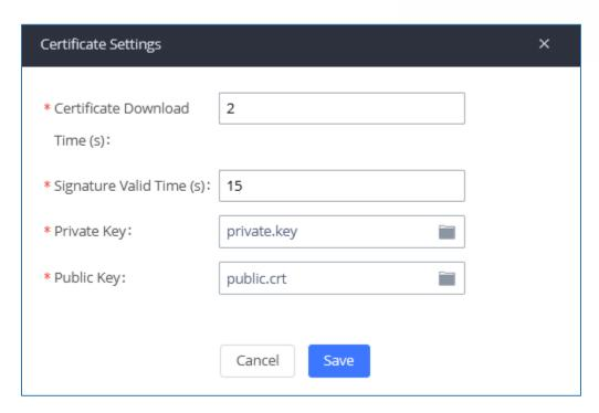
Figure 251: SIP Settings/STIR/SHAKEN – Certificate Settings
