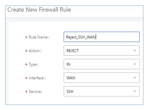
Figure 33: Create New Firewall Rule
