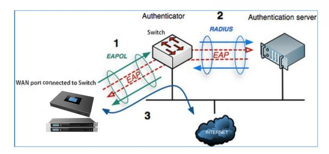
Figure 22: UCM630X Using 802.1X as Client
