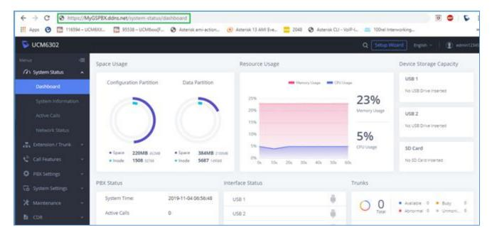
Figure 32: Using Domain Name to Connect to UCM630X
