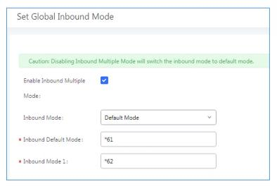
Figure 130: Inbound Route - Multiple Mode Feature Codes
