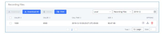
Figure 236: Download Recording File from Recording Files Page
