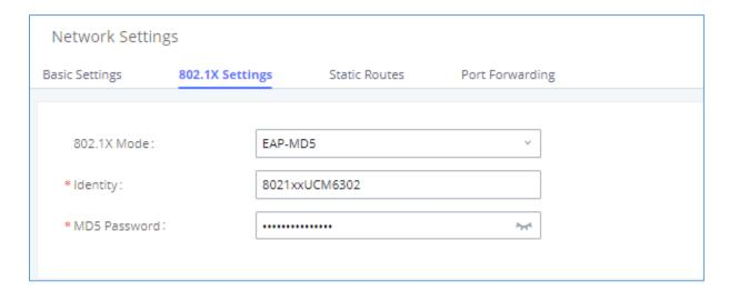
Figure 23: UCM630X Using 802.1X EAP-MD5
