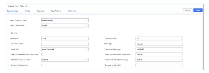
Figure 140: Configure Extension for Fax Machine: FXS Extension
