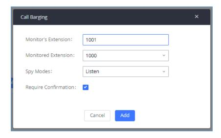
Figure 230: Configure to Monitor an Active Call
