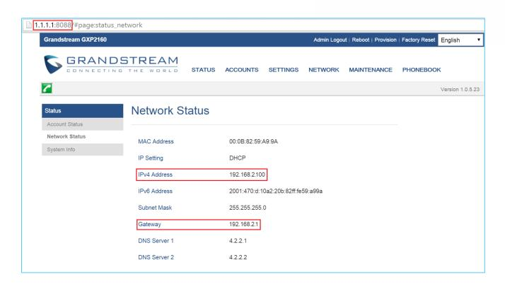
Figure 28: GXP2160 Web Access using UCM6302 Port Forwarding
