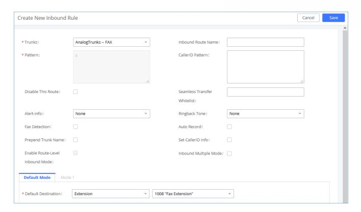
Figure 142: Configure Inbound Rule for Fax
