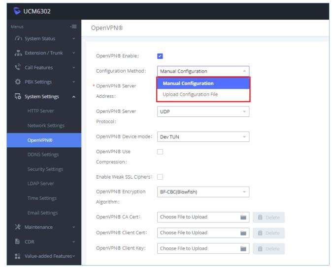
Figure 29: Open VPN® Feature on the UCM630X
