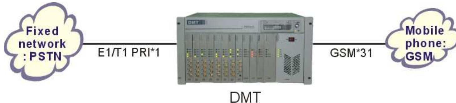
Communication route (it can also provide the reverse direction or bi-direction communication route according to the customer's need)
