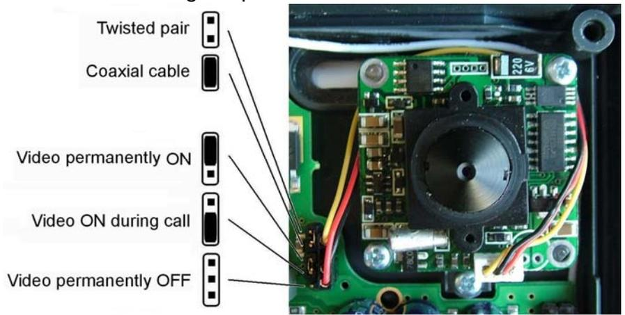
**mode for outdoor installations to avoid camera damage by air humidity.** It is because the camera is heated during operation and thus no moisture condensation can occur.
