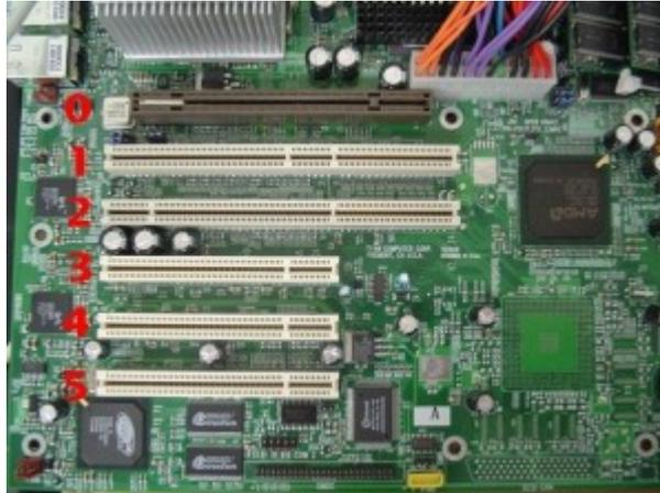
The **TE411P** is a 32-bit 33MHz card keyed for 3.3 volt operation. In the motherboard pictured here, the TE411P will **only** fit into slot #2. The TE411P **will not** fit into slots 1, 3, 4, or 5.
