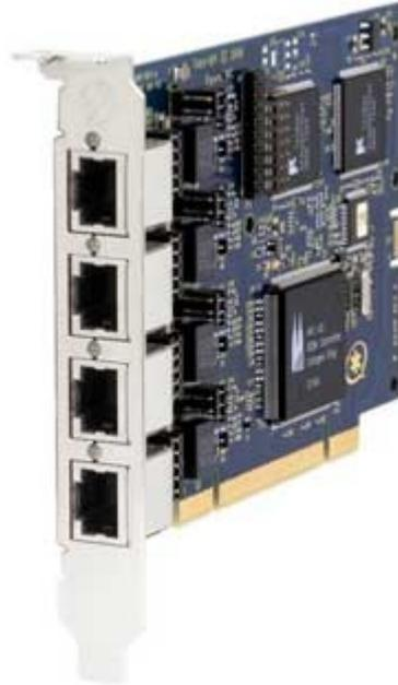
The B410P is a four port BRI card. It supports hardware echo cancellation. **This card is not a zaptel card!** The B410P runs with the mISDN driver from beroNet. For that reason you have to follow the installation instructions in section 3 (3.1 and 3.7). The jumper settings are maybe different from BN4S0, the following picture and table describe the jumpers on the B410P: see next page
