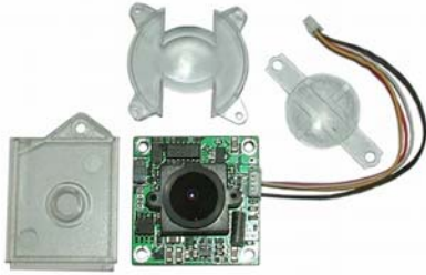
Part No. 9135210E In-built colour CCD camera
