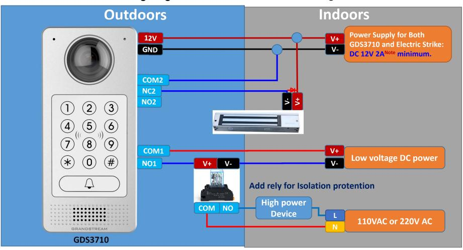
**GDS3710 Connection & Wiring Diagrams ---- Wiegand RFID Reader**
